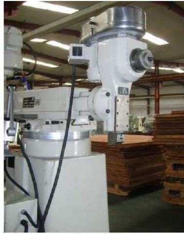
Slotting head with the 0.25KW motor power,
